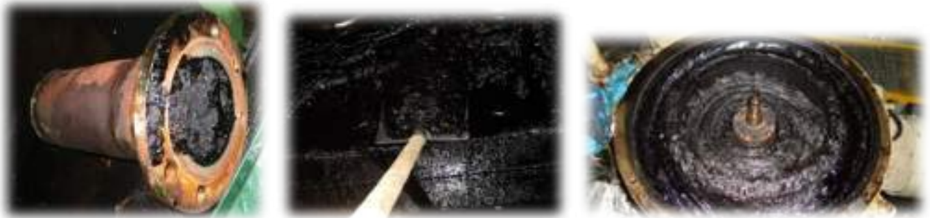
Figure 1: Examples of asphaltene sludge precipitation
